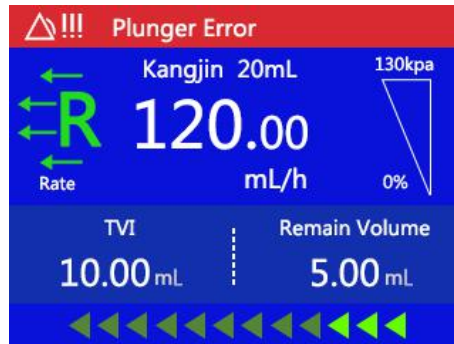
Figure 8-2 Plunger error alarm.
