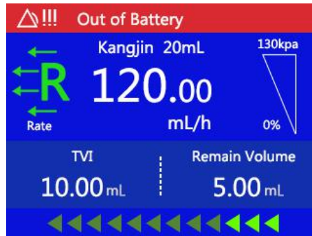
Figure 8-5 Out of battery alarm.
