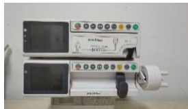
Figure 7-1-2 Stack the Syringe Pump
