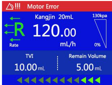
Figure 8-6 Motor error alarm.
