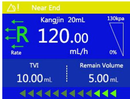
Figure 8-9 Injection near end alarm.
