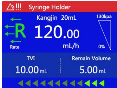
Figure 8-1 Syringe holder error alarm.
