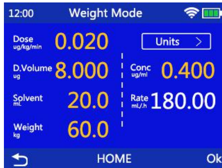
Figure 7-14 -1 Body weight mode setting.
