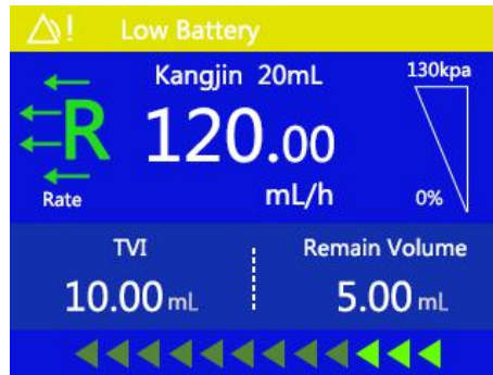
Figure 8-8: Low battery alarm.
