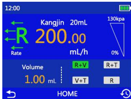
Figure 7-4-1 Identify syringe model
